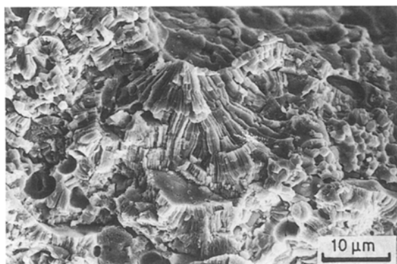
Figure 4 SEM fracture surface of interface with bond layer showing a very fine columnar grain structure for lamellae at the interface.
